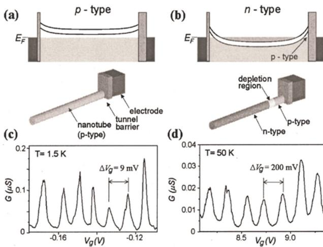
FIG. 2. Band diagrams and schematic pictures of a semiconducting nanotube device when it is field doped (a) *p* type and (b) *n* type are shown. Note that the right-hand side barrier is thicker than the other. (c) Coulomb oscillations are in the *p*-type regime at 1.5 K. The gate period is 9 mV. (d) Coulomb oscillations are in the *n*-type regime at 50 K. The gate period is approximately 200 mV.
