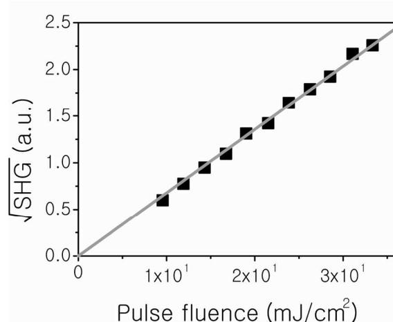
**Figure S4** Incident pulse fluence dependence on the square root of SHG in *h*-BN AB stacking structures.
