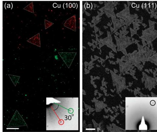
**Figure S1** (a-b) DF-TEM images of *h*-BN sub monolayers grown on (a) Cu (100) and (b) Cu (111) surface. There are two predominant orientations of observed hexagonal diffraction patterns with a 30° angle difference in Fig. S1a, while they are all aligned to a certain direction in Fig. S1b. Scale bar are 200 nm and 2 μm for (a) and (b), respectively.
