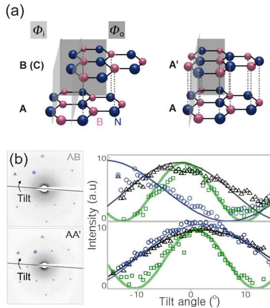
**Figure S2** (a) Schematics of two structural ground states, AB and AA' stacking. Gray boxes indicate diffraction lattice planes for  $\Phi_i$  and  $\Phi_o$  of a diffraction pattern. (b) Diffraction patterns of AB and AA' stackings and intensity changes of three representative spots as a function of the sample tilt angle with respect to the incident beam. Solid lines are calculated from theoretical kinematic diffraction of a 60 keV electron beam.
